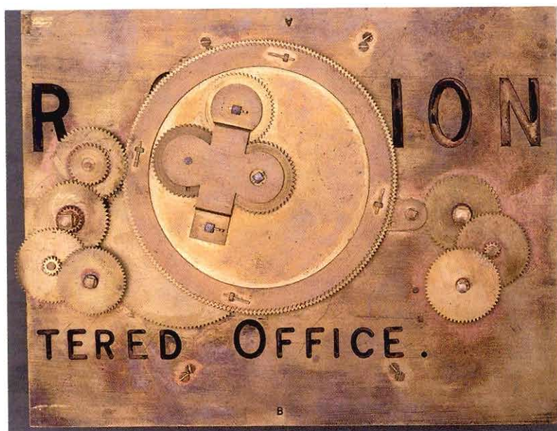
Fig. 6. Model by M.T. Wright, back view of internal frame plate. Compare with figure 5. Note that second-hand materials were used in making this first model, and that some screw-fastenings have been used for convenience in place of rivets.
