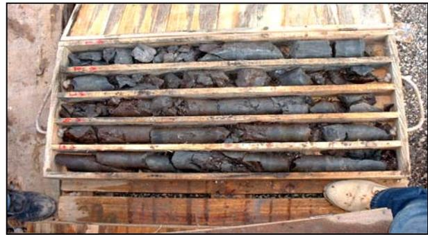
Figure 5. Poor quality flysch (alterations of claystones and siltstones with sandstones intercalations)
