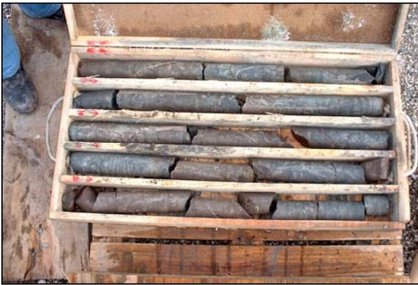
Figure 4. Good quality flysch (claystones, siltstones and sandstones alterations)
