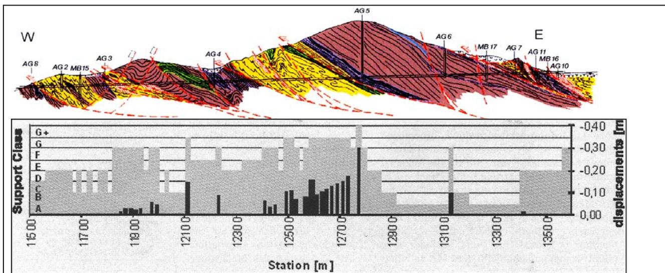
Figure 2. Longitudinal section of Anilio tunnel (from the design; Geology from Mourtzas N & Sotiropoulos E. 1999; support & expected displacements from Schubert W & Riedmueller G 2000)
