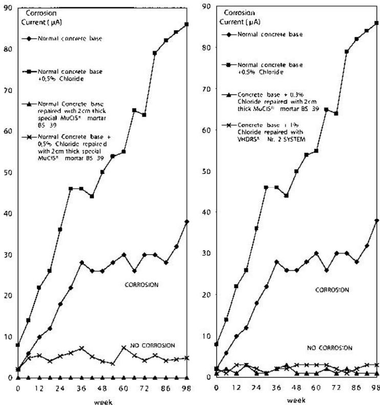
Figure 5: Corrosion current of different systems according to ASTM test G109
