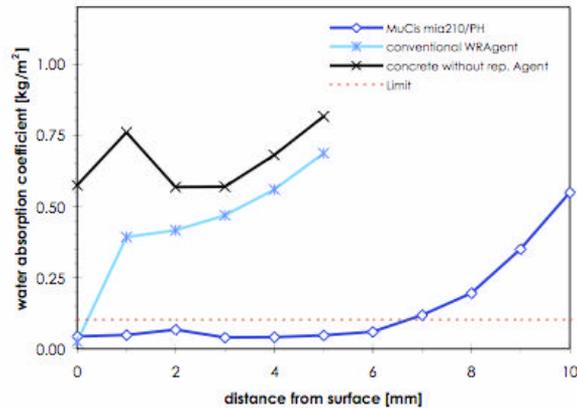
Figure 3: Water absorption profiles of three impregnated concrete and the reference (untreated concrete, w/c=0.55)
