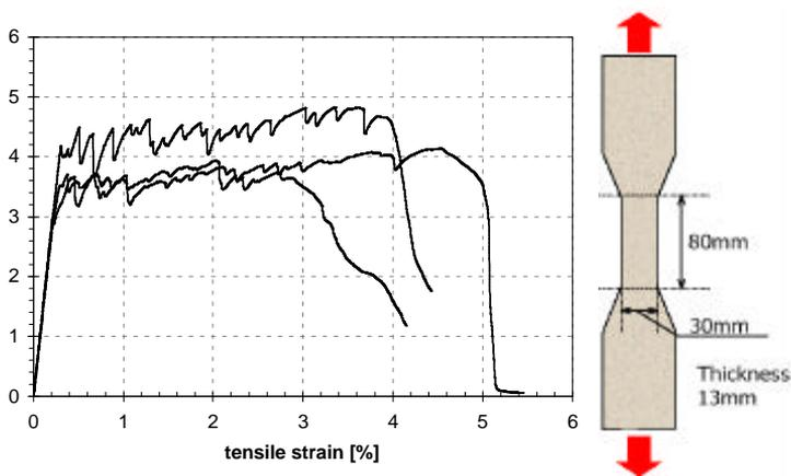
Figure 4: Tensile strain capacity of the described HFE-tec SHCC determined by means of direct tensile tests (3 specimens)
