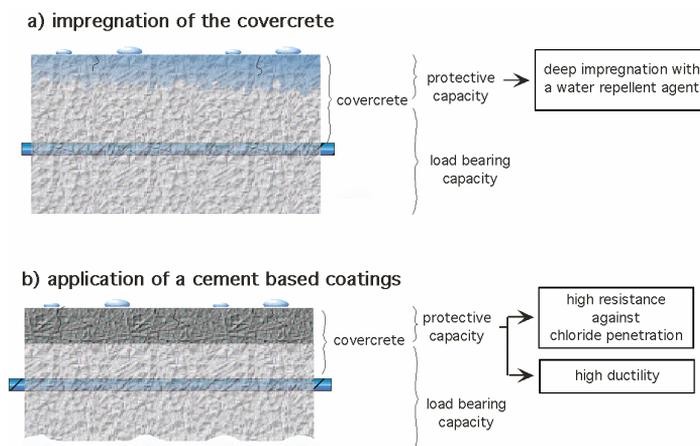
Figure 1: Possible variants for the practical realisation of a multifunctional covercrete a) impregnation of the covercrete b) application of a cement based coating
