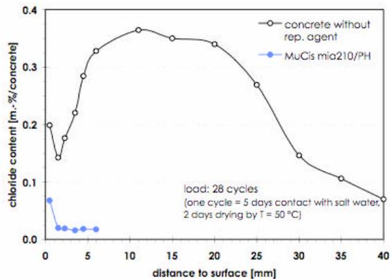
Figure 2: Chloride concentration profiles of a impregnated and the corresponding untreated concrete ( $w/c=0.55$ )
