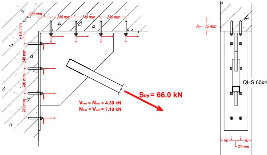
**Figure 6.** Representation of the proposed Brace – Concrete Frame connection. The load of the steel brace as well as the distribution of the loads to each anchor are also noted
