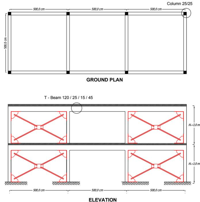
**Figure 5.** Configuration of the analyzed RC Structure retrofitted by use of steel X-Braces
