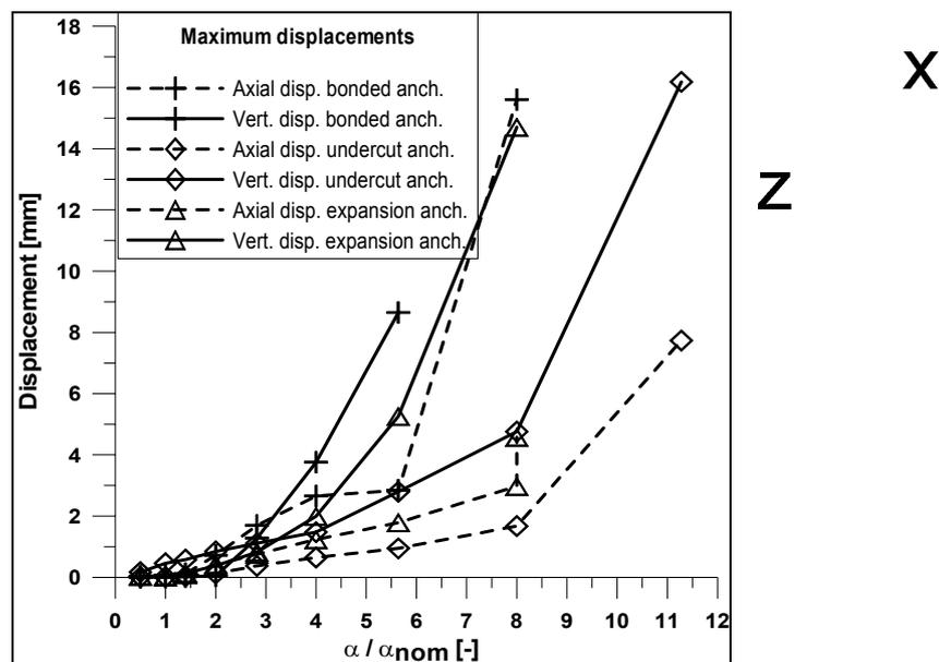
**Figure 4.** Plastic displacements of anchors
