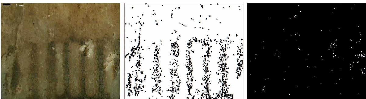
**Figure 7:** (a) Stone material (monitored by a reflectography system (vis)) demonstrating cleaned and un-cleaned stripes, (b) Black particles detected, (c) white particles detected.
