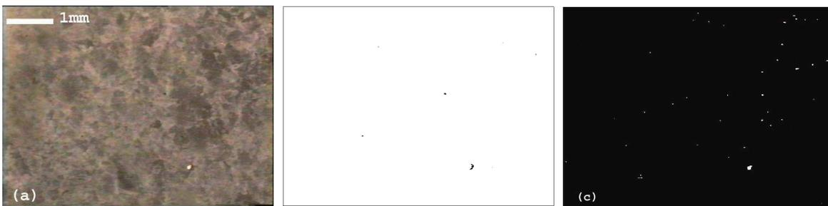
**Figure 5:** (a) Unsheltered untreated Fluting monitored by FOM, (b) black particles detected on (a), (c) white particles detected on (a).
