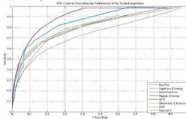
**Figure 8:** ROC curves depicting the performance of the implemented algorithms in the case of the sheltered untreated fluting (illustrated in figure 4).
