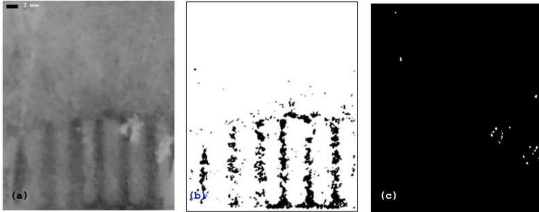
**Figure 6:** (a) Stone material (monitored by a digital camera) demonstrating cleaned and un-cleaned stripes, (b) Black particles detected, (c) white particles detected.
