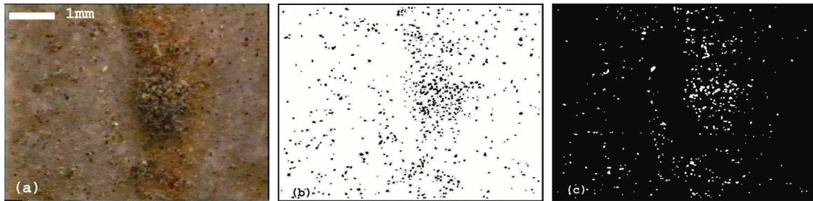
**Figure 4:** (a) Sheltered untreated Fluting monitored by FOM, (b) black particles detected on (a), (c) white particles detected on (a).
