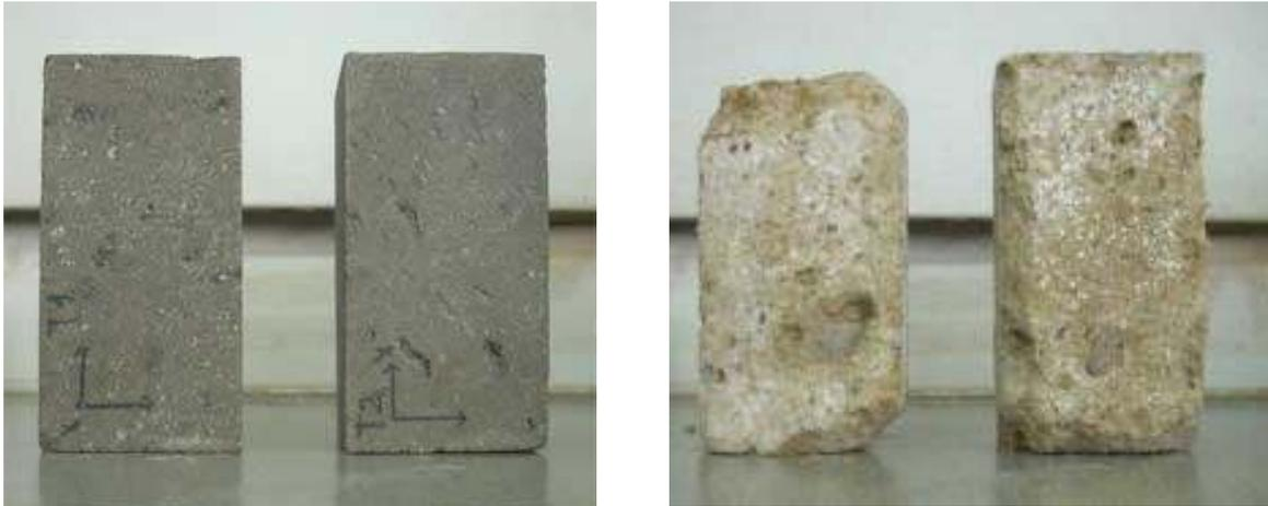
**Figure 8:** Specimens of CI grey (left) and yellow (right) facies treated with consolidant at the end of SWT2 test
