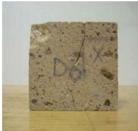
**Figure 5:** Crack net occurring after WDT on a CI yellow facies sample treated with T-CON
