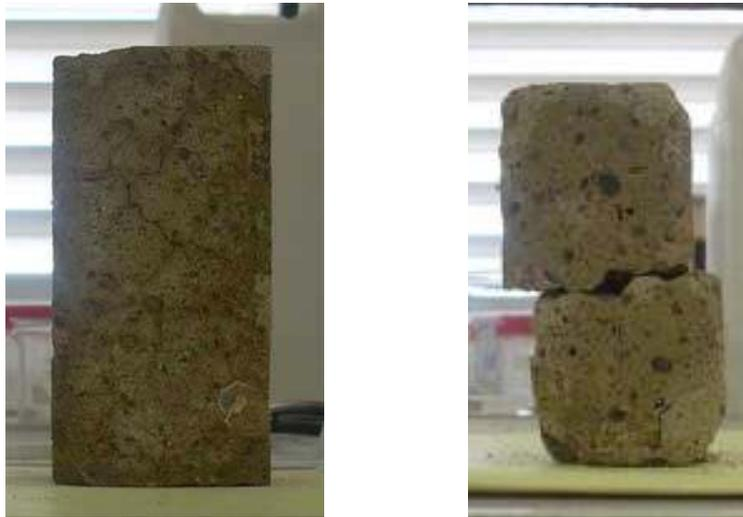
**Figure 7:** Specimens of CI yellow facies after 1 cycle (left) and at the end of SWT1 (right)
