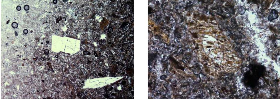
**Figure 3:** Polarized light micrographs of CI grey facies (left) and yellow facies (right)
