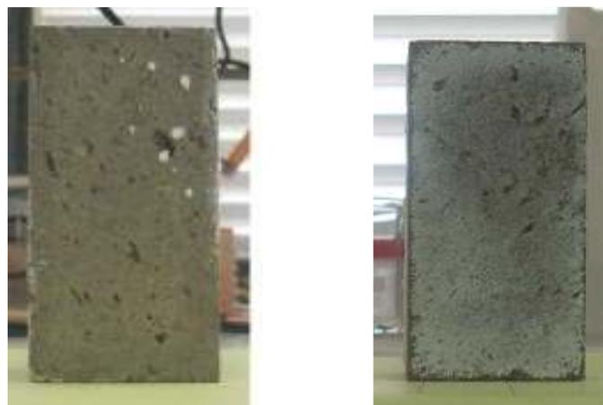
**Figure 6:** Specimens of CI grey facies after 2 cycles (left) and at the end of SWT1 (right)
