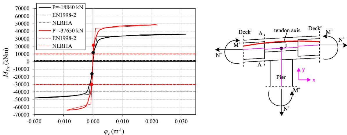
Fig. 1 Moment-curvature curves (flexure about z axis) of deck section A-A under different levels of prestressing force compared with the deck ‘capacity design’ moments (dashed lines) obtained from EN1998-2 and the NLRHA-based approach
