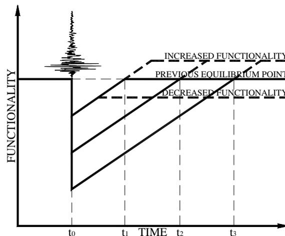
Fig. 2 Recovery after an earthquake, functionality variable with constant recovery rate,  $t_0$  to  $t_1$ ,  $t_0$  to  $t_2$  and  $t_0$  to  $t_3$  are possible measures of resilience
