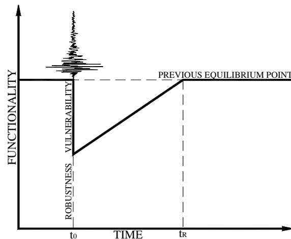
Fig. 1 Recovery after an earthquake
