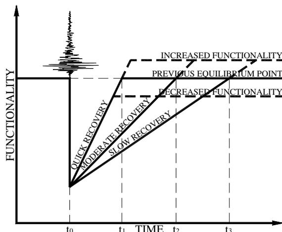
Fig. 3 Recovery after an earthquake, recovery rate variable,  $t_0$  to  $t_1$ ,  $t_0$  to  $t_2$  and  $t_0$  to  $t_3$  are possible measures of resilience
