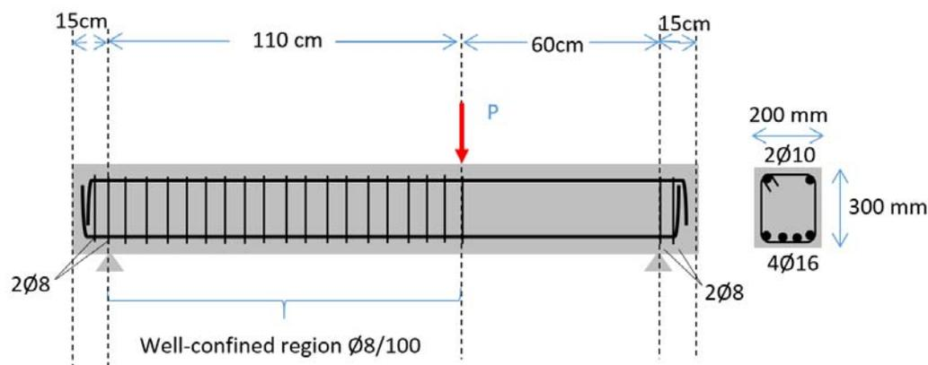
Fig. 1 Beam geometry and reinforcing details.
