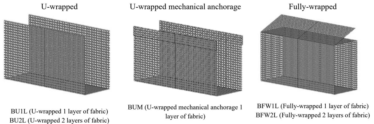
Fig. 3 SRG jacket configurations
