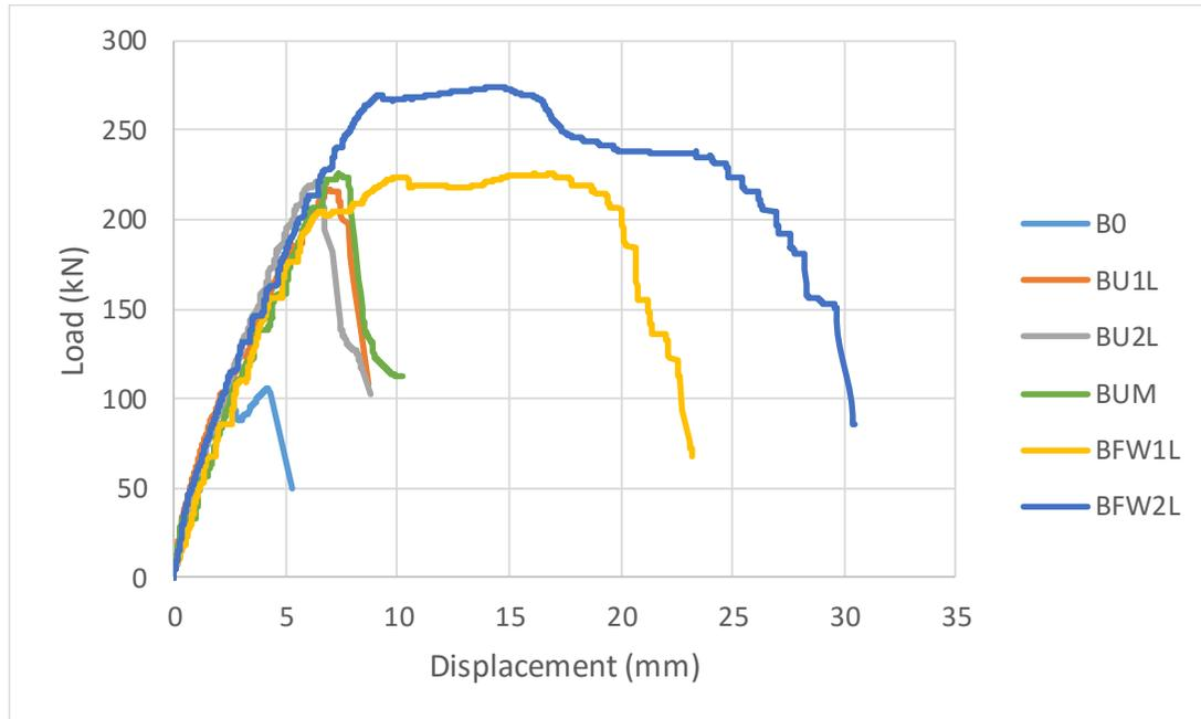
Fig. 4 Load versus vertical displacement curves for all tested specimens.
