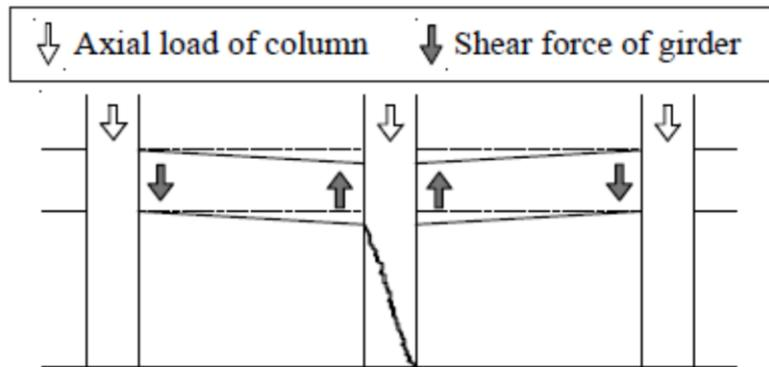
Figure 1: Mechanism of axial load increase of columns neighbouring an axially failing column. (taken from Nakamura & Yoshimura, 2014)
