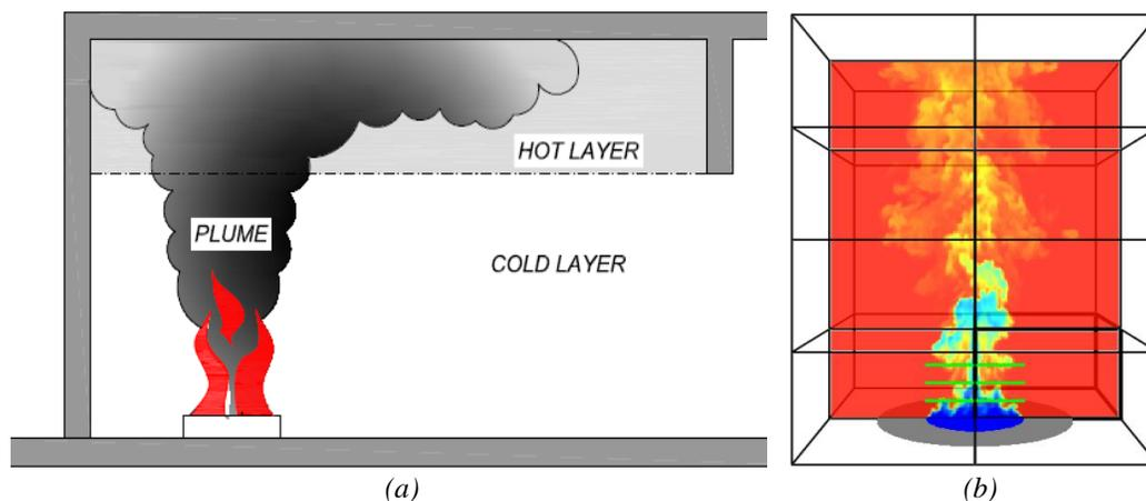
Fig. 1 a) Concept of a two-zone model b) CFD model [3]
