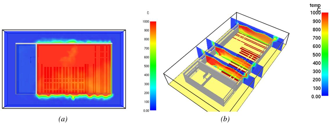
Fig. 4 a) Temperature distribution under the roof b) Temperature distributions in the compartment
