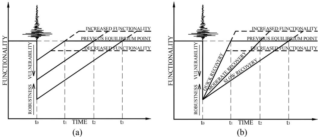
**Figure 1.** Recovery after an earthquake, (a) loss of functionality variable with constant recovery rate and (b) recovery rate variable ( $t_0$  to  $t_1$ ,  $t_0$  to  $t_2$  and  $t_0$  to  $t_3$  are the times taken to recover from a destructive earthquake)
